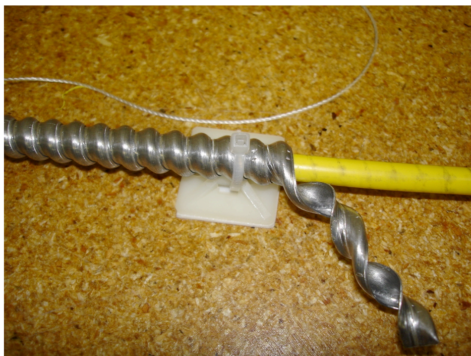
Figure 3. Partially unwrapped armor illustrating continuous wrap
