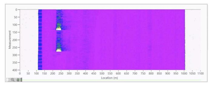
The resulting data sets are resolved into two dimensions: Time and Distance. Each sample point behaves like a two-path interferometer. The signal is then passed through ML signal processing algorithms for event generation. This processing allows for precise identification of the location and type of threat.
